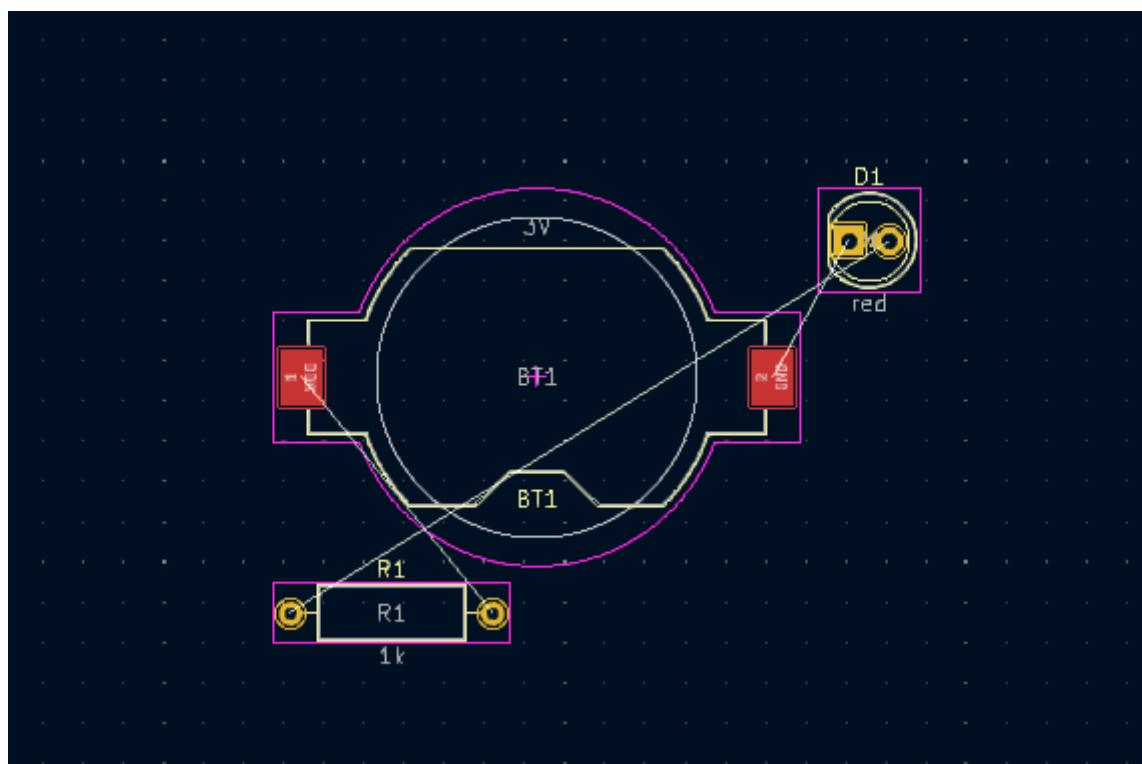
In KiCad, updating the PCB with changes in the schematic is a manual process: the designer decides when it is appropriate to update the PCB with modifications in the schematic. Each time the schematic is edited, the designer must use the **Update PCB**
