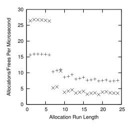
Figure 6.21: Allocator Cache Performance
