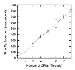
Figure 5.1: Atomic Increment Scalability on Nehalem
