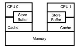
Figure 15.1: System Architecture With Store Buffers
