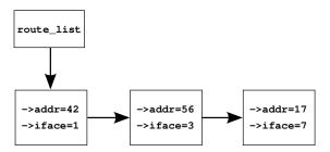
Figure 9.1: Pre-BSD Packet Routing List
