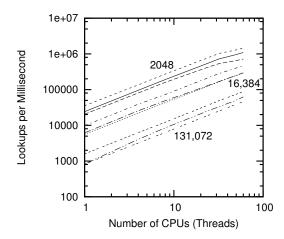
Figure 10.17: Overhead of Resizing Hash Tables
