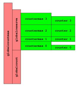
Figure 5.5: Simple Limit Counter Variable Relationships
