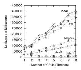
Figure 9.16: Pre-BSD Routing Table Protected by RCU QSBR
