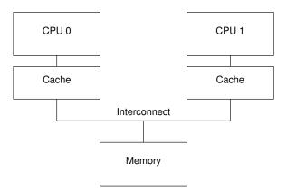
Figure C.1: Modern Computer System Cache Structure
