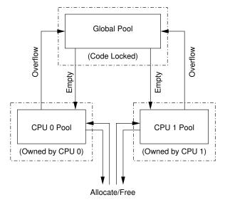
Figure 6.19: Allocator Cache Schematic
