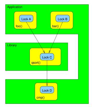
Figure 7.6: Layered Locking Hierarchy for qsort()
