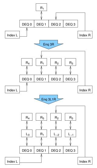
Figure 6.8: Hashed Double-Ended Queue After Insertions
