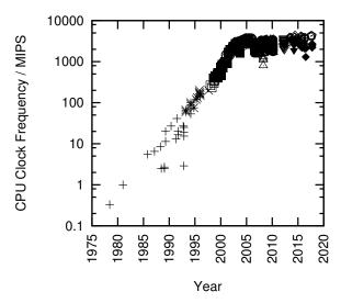
Figure 2.1: MIPS/Clock-Frequency Trend for Intel CPUs
