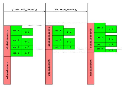
Figure 5.6: Schematic of Globalization and Balancing
