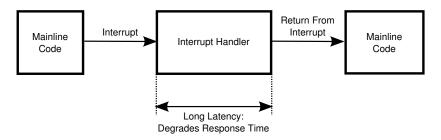
Figure 14.12: Non-Threaded Interrupt Handler
