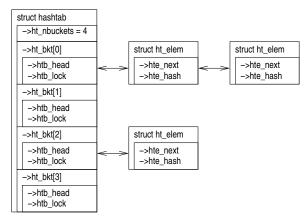
Figure 10.1: Hash-Table Data-Structure Diagram
