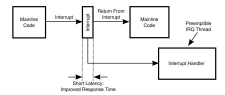
Figure 14.13: Threaded Interrupt Handler
