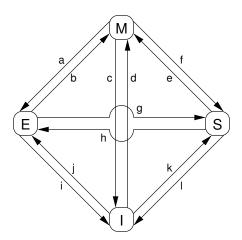
Figure C.3: MESI Cache-Coherency State Diagram
