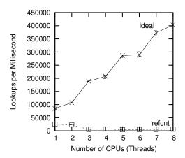
Figure 9.2: Pre-BSD Routing Table Protected by Reference Counting
