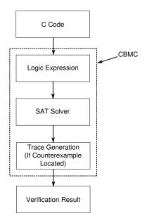
Figure 12.2: CBMC Processing Flow
