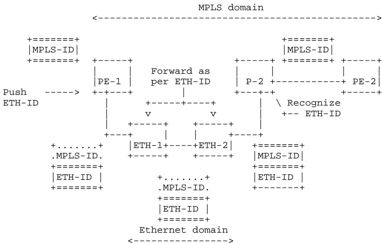
Figure 11: MPLS nodes interconnected by an Ethernet domain
